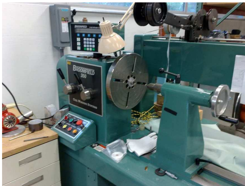
Figure 5.5: the Broomfield winding machine.
