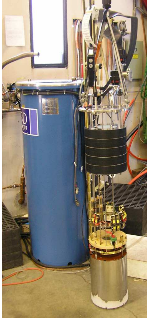
(b) superconducting magnet system of the Tesla-tron II, removed from its cryostat.
