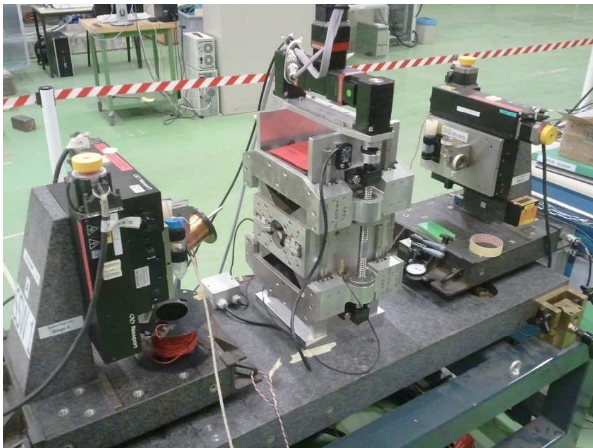
Figure 1: stretched wire measurements set-up.
